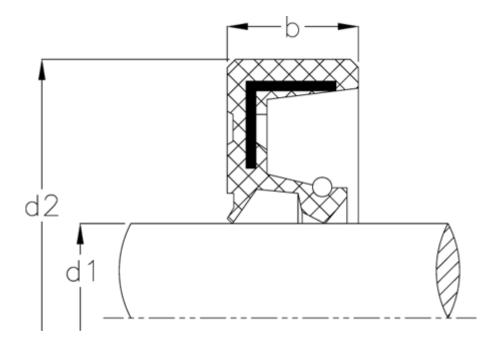
$\begin{array}{ll} b & = 10 \\ d1 & = 30 \\ d2 & = 47 \\ Material = NBR \end{array}$
